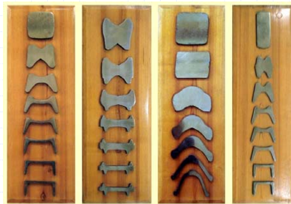
Cross-sections of continuously rolled structural shapes, showing the change induced by each rolling mill
