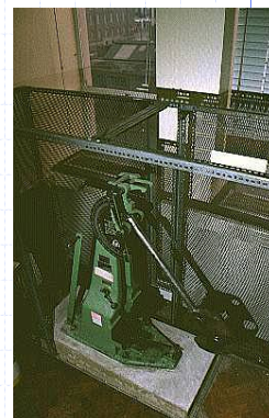
Testing equipment - Charpy's hammer
