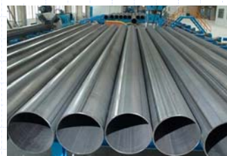
Seamed tube finished product (no weld is visible)
