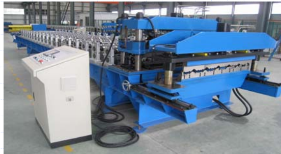
Cold forming of steel metal decking
